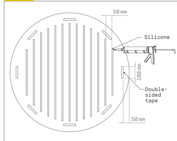
Cut 100 mm strips of double-sided tape and apply 50 mm in from the edge of the mirror as per diagram.
